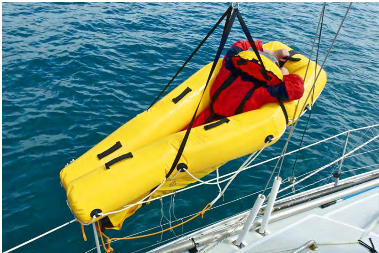
Image 2.7 Pulley device lifts user from the water comfortably
