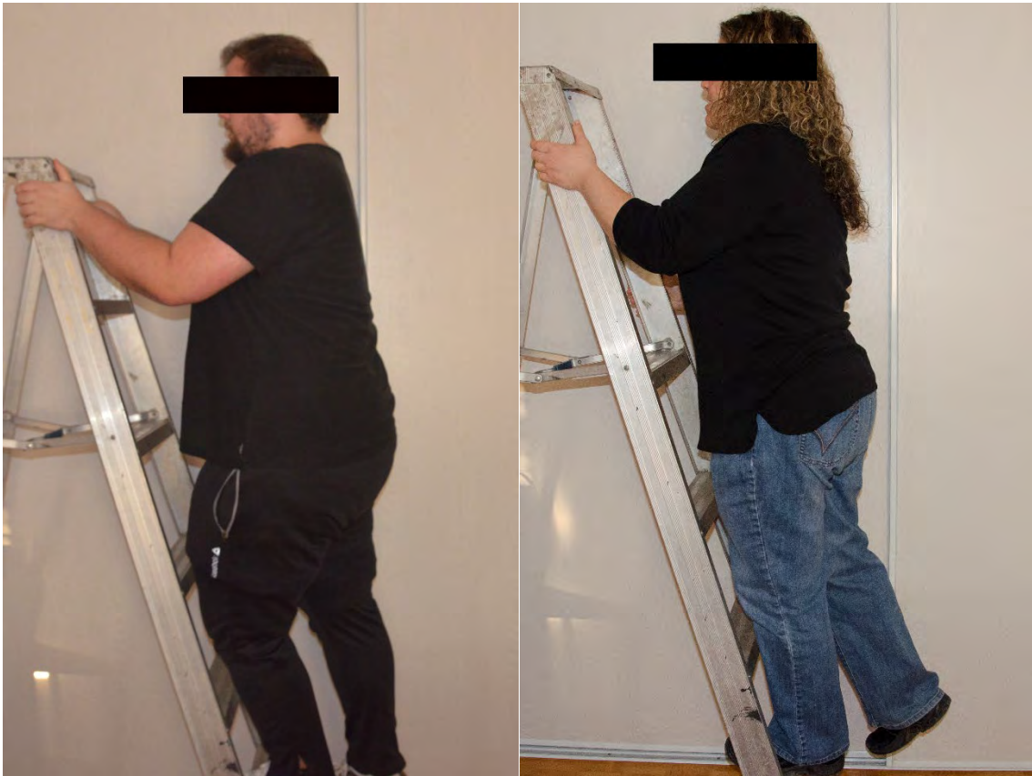
Figure 3.9 Test 4: 95 th & 5 th percentile interaction
