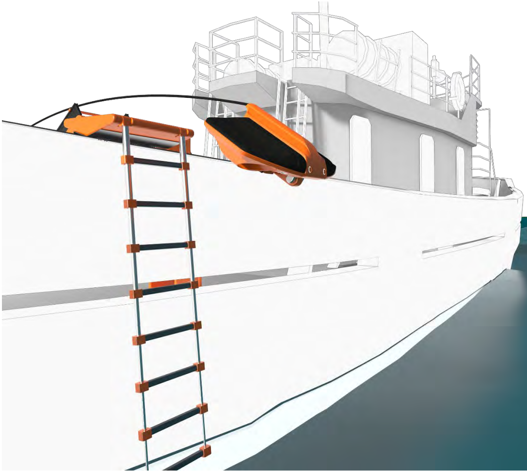
Figure 5.5 Retrieval Device Launch from Vessel
