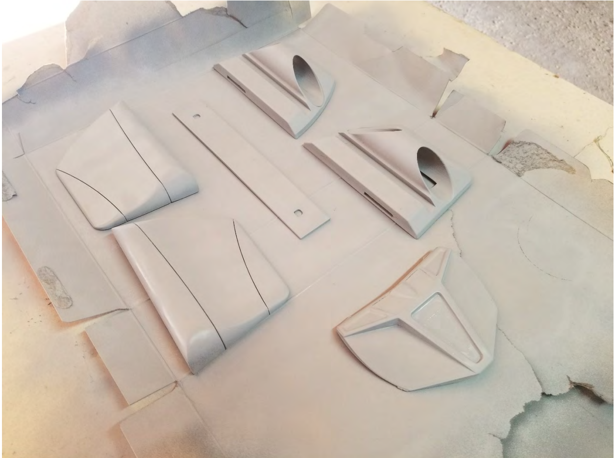
Figure 4.24 after a few coats of filler primer the parts were sanded again to create a smooth surface for the top coat of paint
