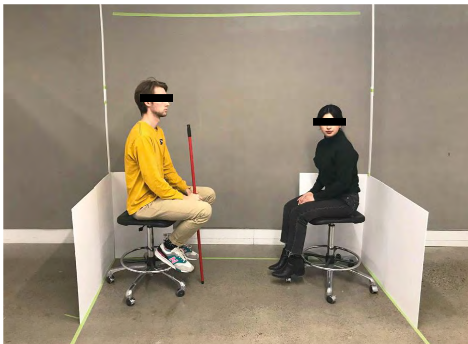
Figure 3-7: 95th percentile male and 5th percentile female sitting inside fishing platform buck model
