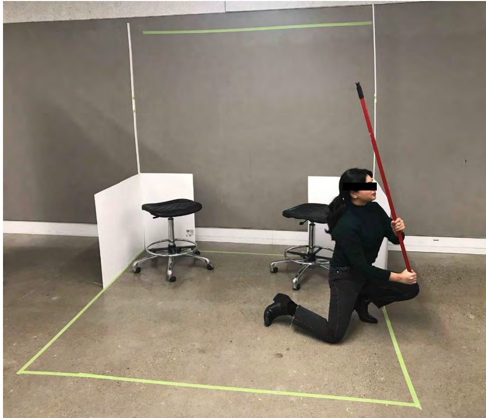
Figure 3-8: 5th percentile female kneeling with buck model fishing rod and pretending to reel
