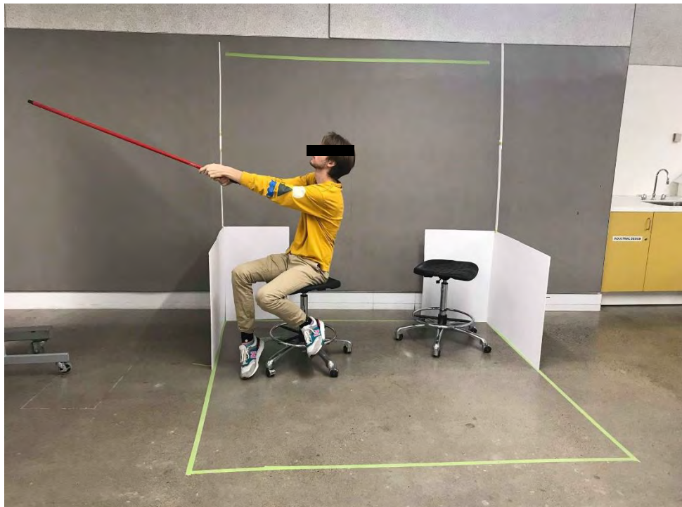
Figure 3-9: 95th percentile male sitting and casting the buck model fishing rod for measurements regarding space
