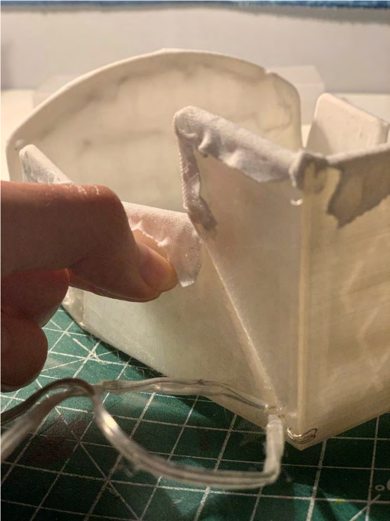
Figure 49 - Inside fabric - glue sprayed and wrapped on the sides
