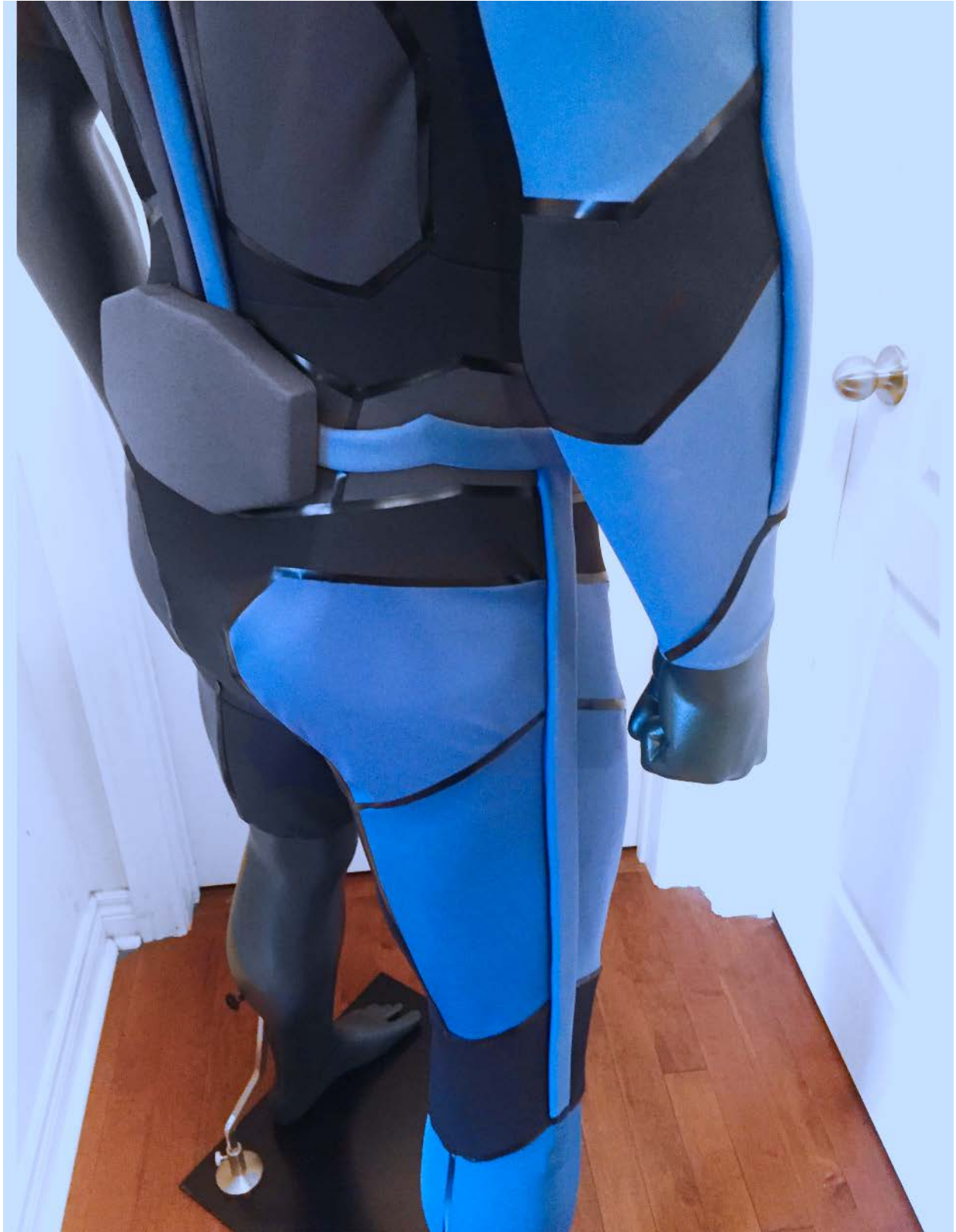
Figure 45. Wire Casing Terminates Into Exterior Shell
