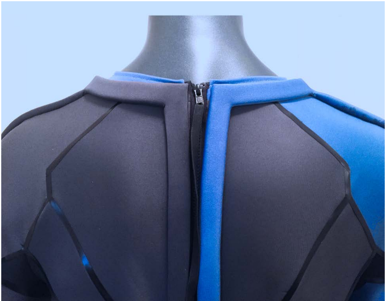
Figure 46. Wire Casing Runs Along Entrance Zipper
