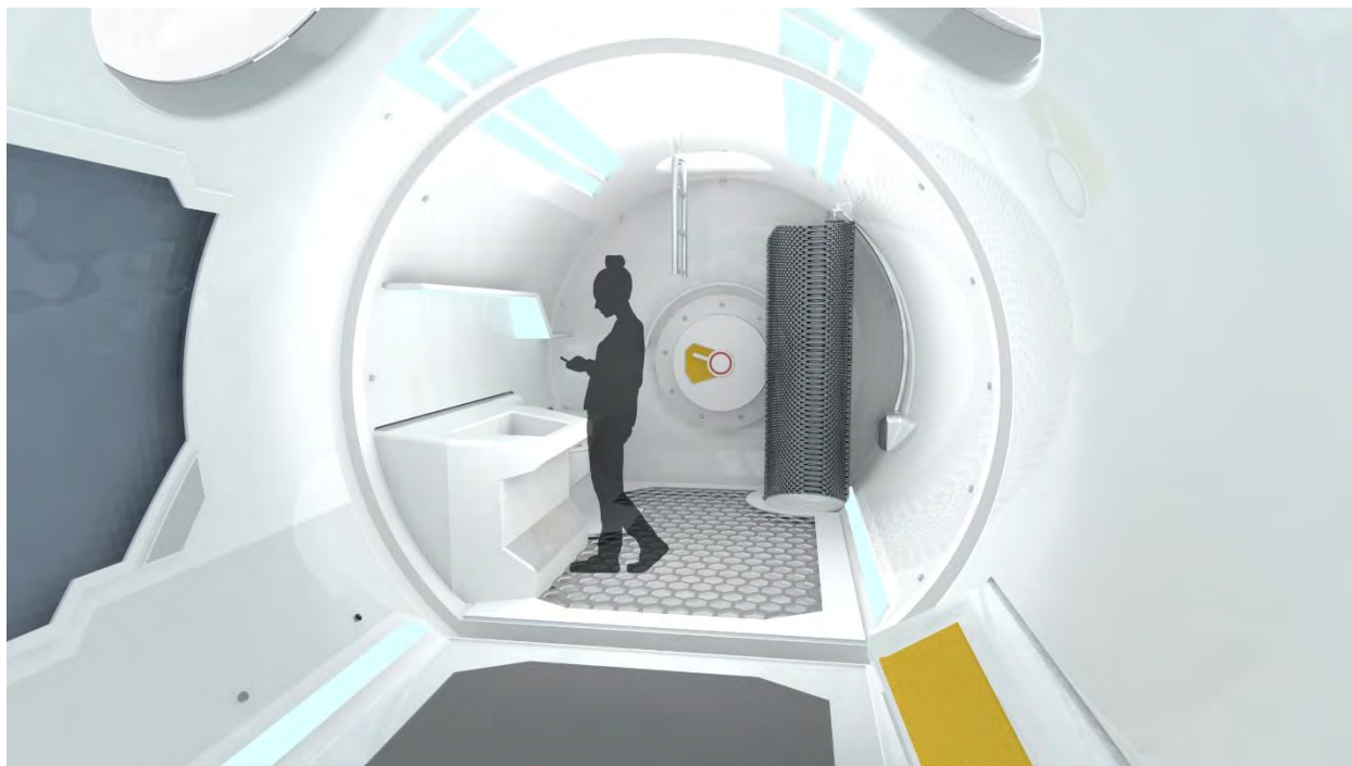
Figure 35 – Interior view of ablution area. Contains shower and privacy mesh, sink and toilet.
