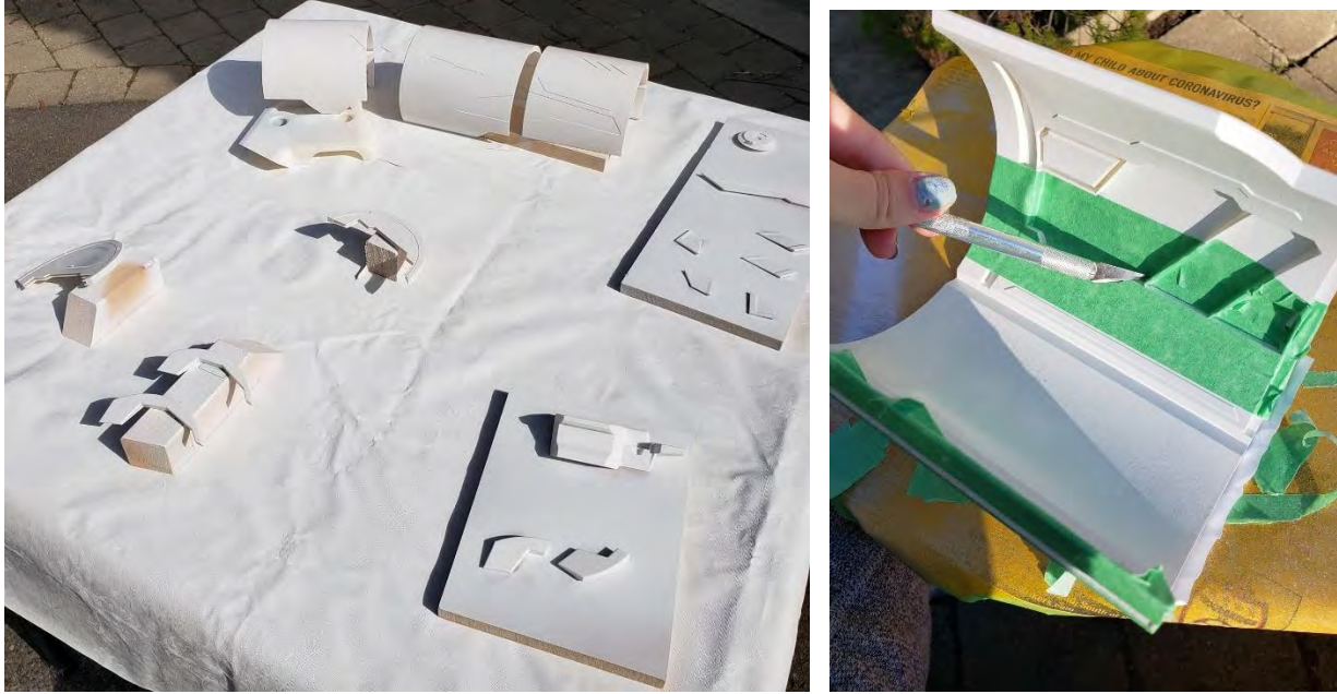
Figure 31 - Hard Model Fabrication - Parts were set up to be primed, sanded and painted with a gloss white coat. Masking was done to achieve alternate colours in detailed areas.
