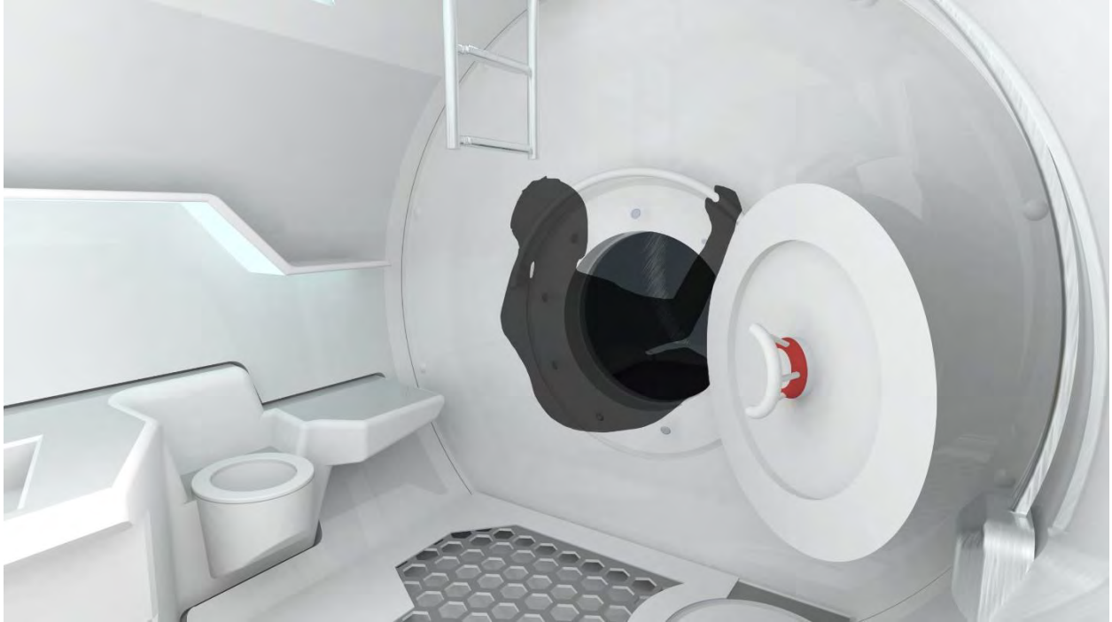
Figure 43 – Divers Weight is supported to enter or exit the dive bell by semi-circular grab bar.
