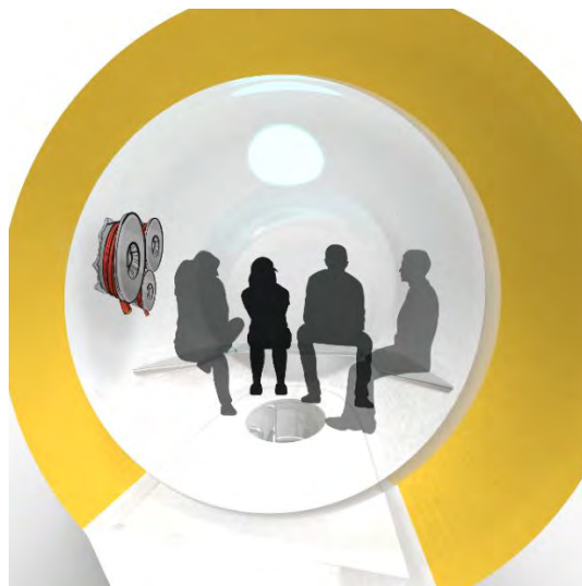
Figure 39 – Interior view of dive bell. Shows four divers preparing to submerge underwater. Umbilical chord for oxygen and heat are installed on the left hand side.
