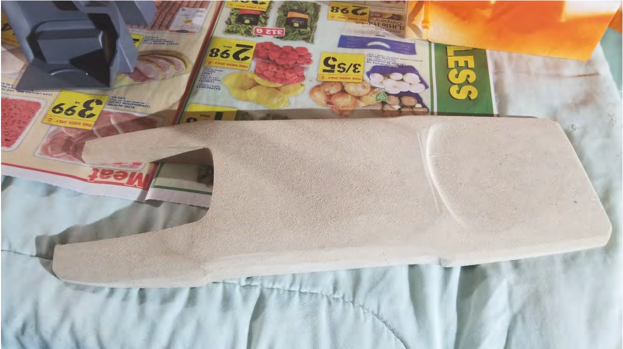
Hand fabricated roof piece out of laminated MDF. Original plan was to CNC from Renshape however due to Covid-19 and time restrictions it was the resorted plan.
