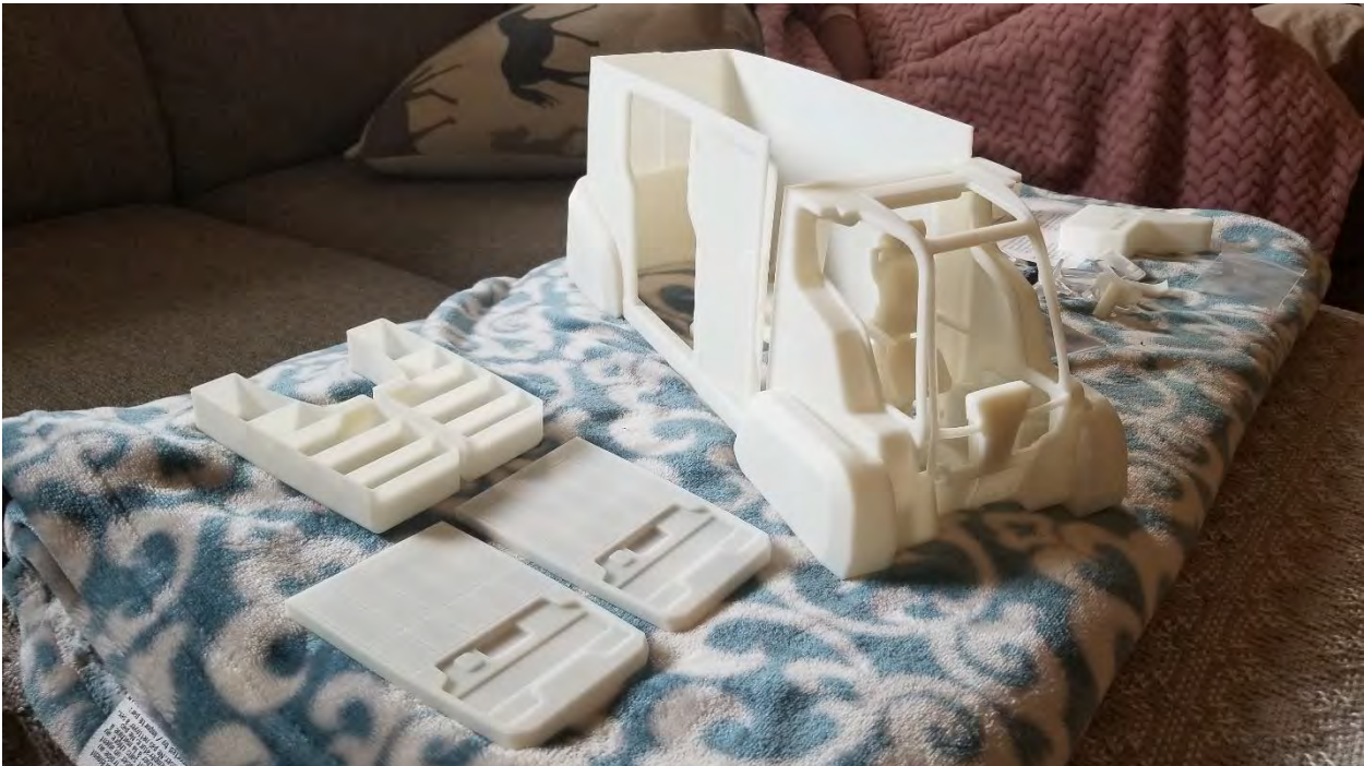
Dry fit of 3D printed parts.
