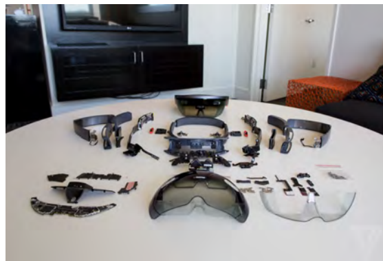
Figure 3-9-1 – Teardown of the Microsoft HoloLens V1. Photo by The Verge
