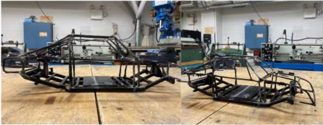
Assembly/Finishing: Sanding, Grinding and Painting Roll-Cage
