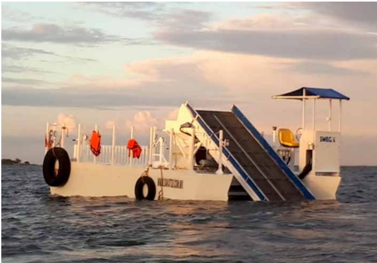
Figure 8 shows the SWS75 sargassum collector boat from the Techno Products Gab company. This picture was retrieved from: https://www.tecnogab.com.mx/sws75
