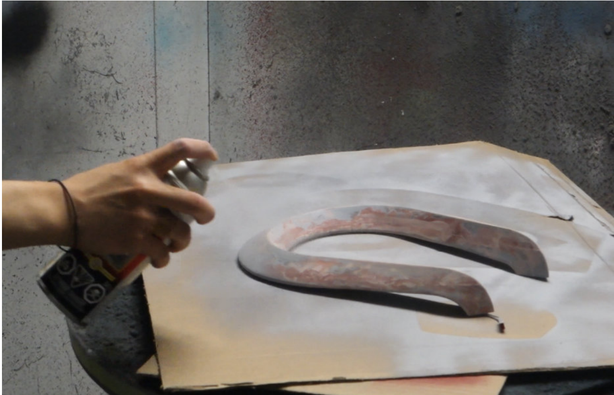
Figure 60 – Priming the Sanded Top Portion of the Ring
