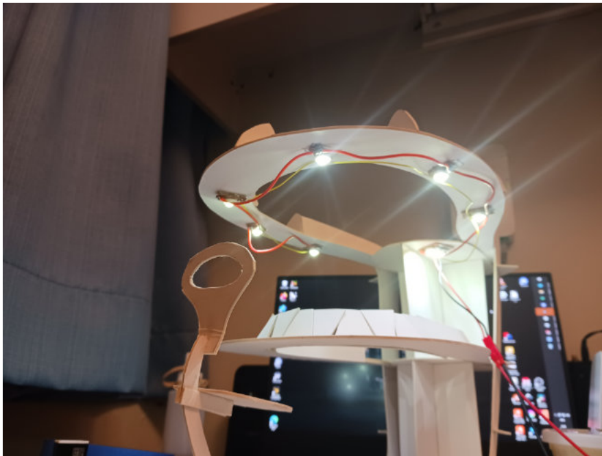
Figure 45 – 10:1 Scale Model With Lighting Circuit Installed
