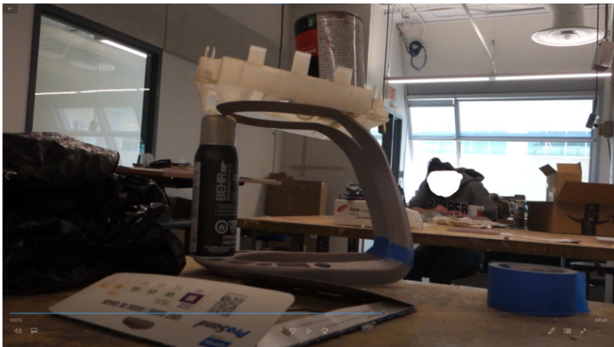
Figure 56 – Epoxying the Three Different Parts That Made Up the Ring
