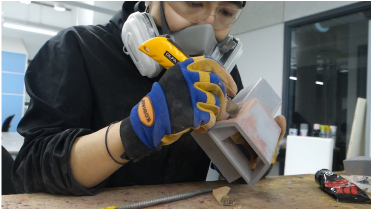
Figure 55 – Removing Support Material and Filling Gaps with Glazing Putty
