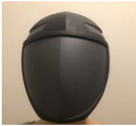
Figure 76. 3D Printed Helmet - Spray Painted
