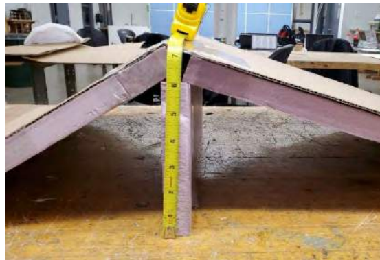
Figure 24 - A Measurement of the Knee Bend and Basic Construction (7.5" High)
