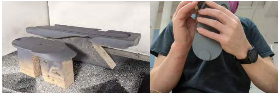
Figure 92 - SLA parts were primed and wet sanded, then painted
