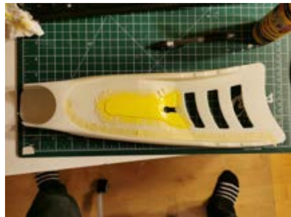
Taping off of areas that don't need to be painted
