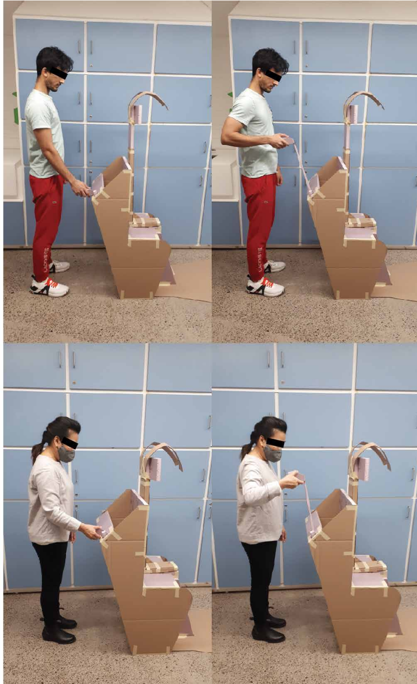
Figure 14: 99th percentile male (top) and 50th percentile female (bottom) testing ergonomic dimensions of the club rack height. Subjects are shown grabbing a club at the rack (left) and lifting it out (right).
