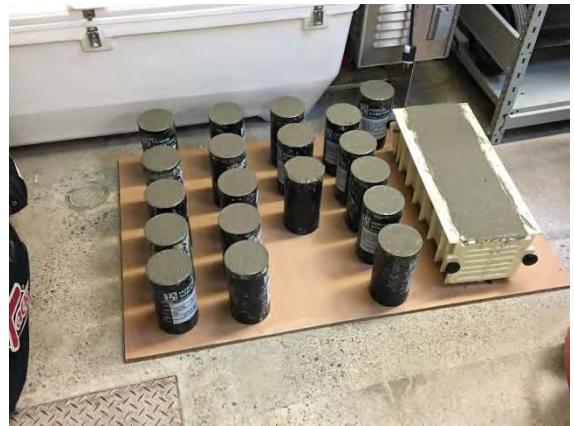
Figure 4 - Casting of Molds
