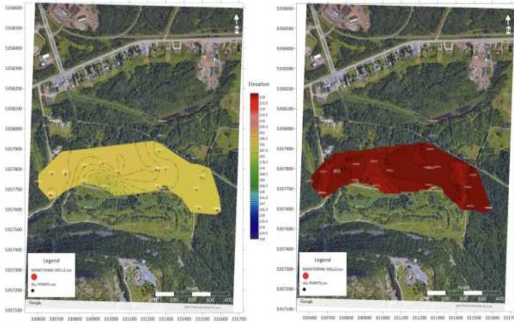
Figure 57. In the left, the contour map and in the right isopach map of the layer peat.
